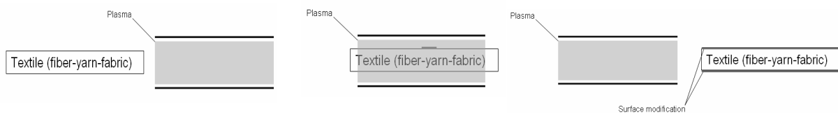
Fig 1 a (left), b (centre) and c (right) showing substrate undergoing surface modification as it passes through plasma.
